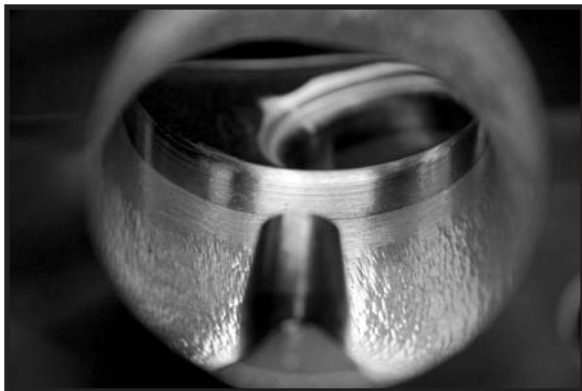
Intake Port and Polished Seat
